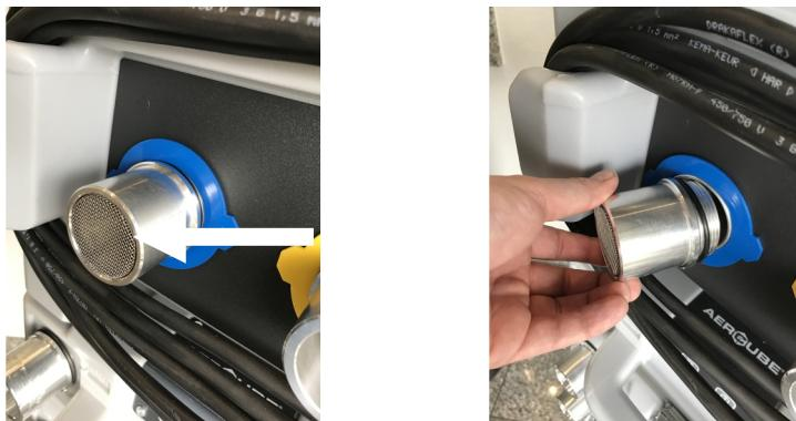
Fig. 9: Coarse filter intake socket
