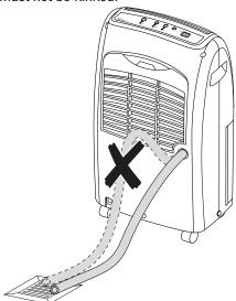
Remove the hose if you want to collect the condensate in the condensation tank again. Allow the hose to dry prior to storage. The hose can be connected in any operating mode for continuous operation.
