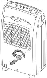
2. Remove the condensation tank.
