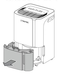
2. Empty the condensation tank into a drain or sink.
