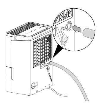
Guide the other hose end to a suitable drain or sufficiently dimensioned collection container. Please note that the hose must not be kinked.
