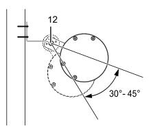
8. Once the device is at the desired inclination angle, tighten both Allen screws (12) again.
