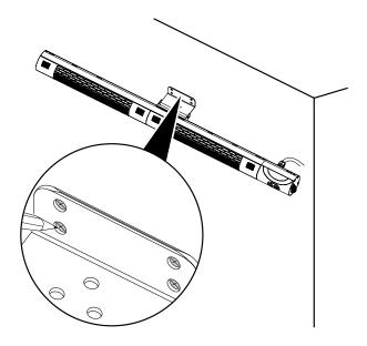
2. Drill the drill holes into the wall at the marked positions.
