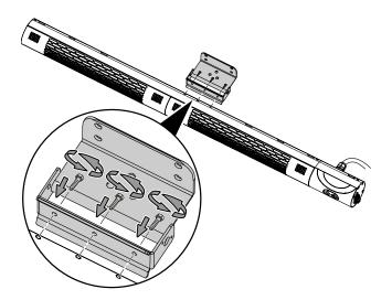
2. The position of the holder can be freely adjusted.
