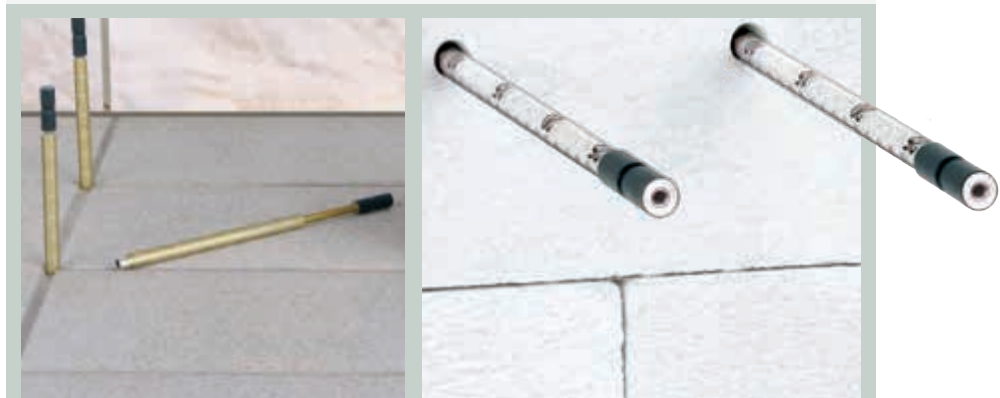
DETAIL Both electrode pairs are equipped with one-centimetre division scale
