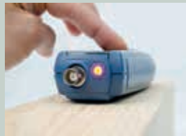
Non-destructive measurement by means of a single-point contact area [LED flashing signal for limit crossings]
