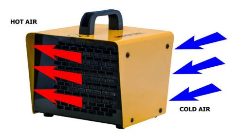
The device works on the principle of forced convection. The airflow is forced by fan. The cold air is sucked in at the rear of the unit. The cold air becomes heated when flow through the PTC heating element. The heated air exits the front of the heater. The device can heat a half or full power. The device is equipped with thermal protection running automatically. The device has a thermostat for adjusting temperature in the range 0°C - 40°C.
