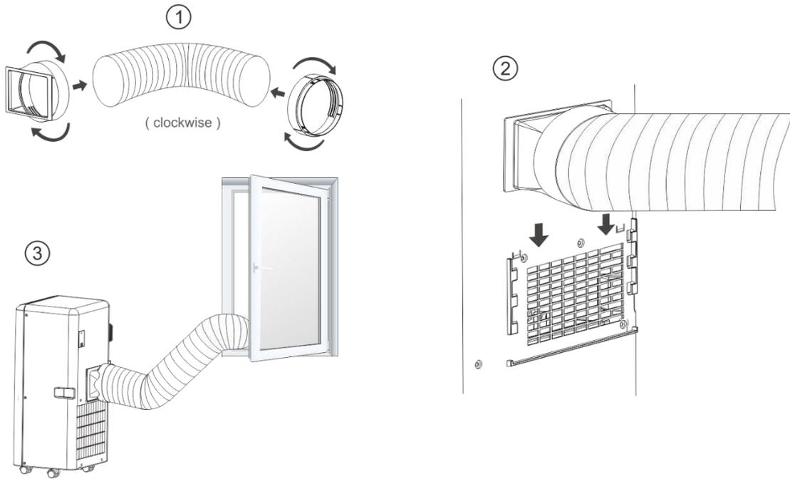
Fasten the exhaust air connection to the exhaust air hose. (1) Now attach the exhaust air hose to the unit. (2)
