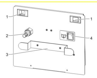
Fig. 5: Pump-out kit for air dehumidifier AD 740
